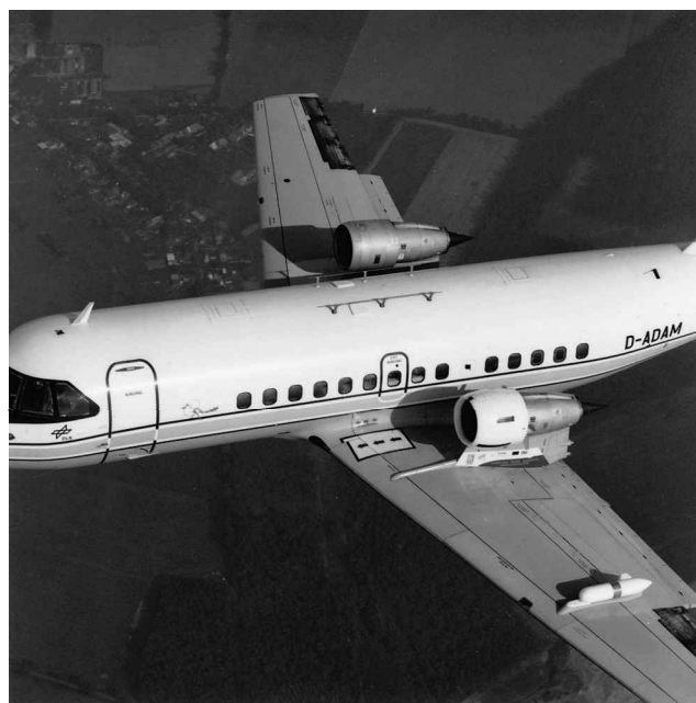
Fig. 3 VFW614/ATTAS in-flight with the NLF nacelle installed on the port engine.
